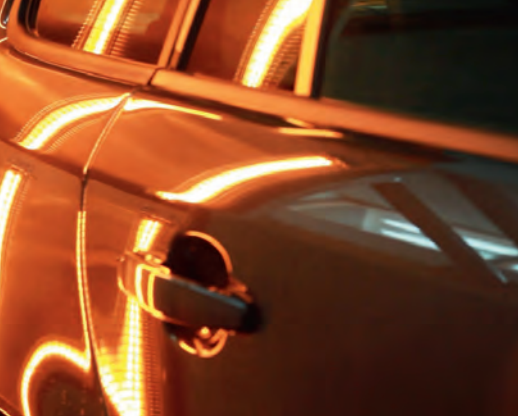
The shape and positioning of the reflectors give an even heat distribution.
