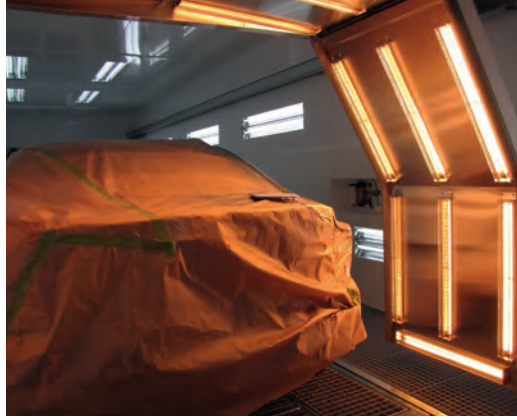
The IRT PowerCure automatically moves to the right position corresponding to the chosen panels.
