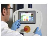
**Booth VS6:** control panel with colored touch screen, navigation icons, scroll-down menus, automation of functions, PLC centralised management.
